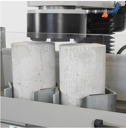
Specimen grinding machine 55-C0202 with locking system for two concrete cylinders (55-C0200/160 and 55-C0200/1602)
